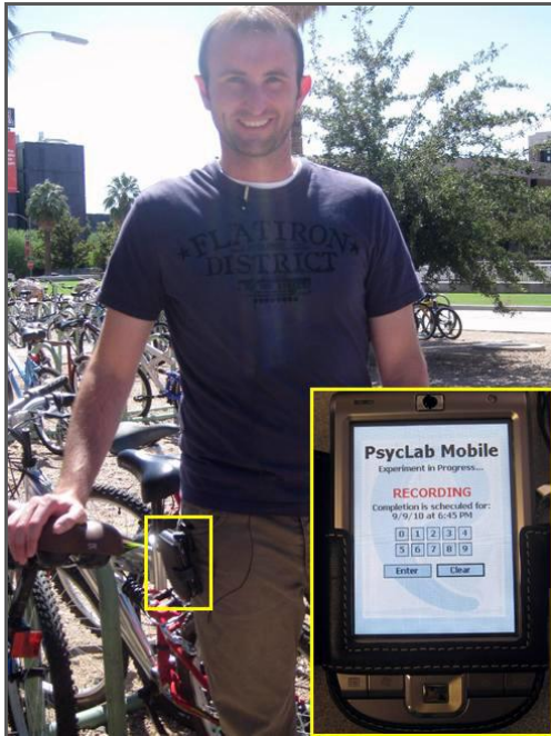
Figure 12.2. Picture illustrating how the PDA-based EAR-system is worn by a person.
